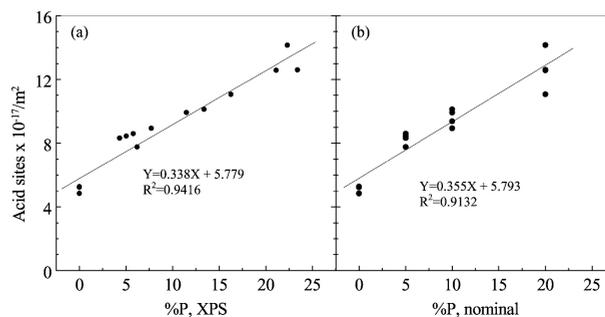
**Fig. 10** Relationship between the number of acid sites per  $\text{m}^2$  and the (%P) on the surface as determined by XPS (a) and the (%P) of the nominal composition of samples (b) (eqn. (7) and (8) respectively).
