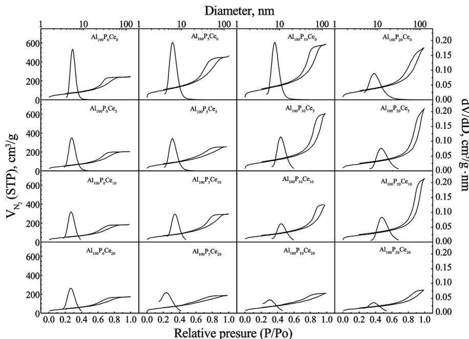
Fig. 2 Adsorption-desorption isotherms (77 K) of Al-P-Ce-O mesoporous solids and the corresponding pore size distribution (BJH).
