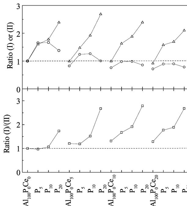
**Fig. 8** Upper part: ( $\Delta$ ) Ratio I (eqn. (3)) of the surface acidity of each  $\text{Al}_{100}\text{P}_X\text{Ce}_Y$  sample over the surface acidity of the parent sample  $\text{Al}_{100}\text{P}_0\text{Ce}_0$ ; ( $\circ$ ) Ratio II (eqn. (4)) for SSAs. Lower part: ( $\square$ ) the ratio (I)/(II) showing the relative increase in acidity compared to the increase in surface area. The dotted horizontal lines at the point 1 are a guide for the eye.
