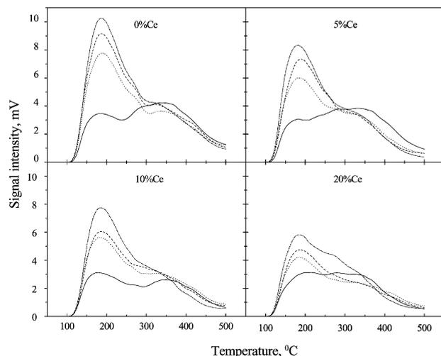
**Fig. 4**  $\text{NH}_3$  TPD signals of the  $\text{Al}_{100}\text{P}_x\text{Ce}_y$  solids. 0%P (solid line), 5%P (dotted line), 10%P (dashed line) and 20%P (dashed-dotted line).
