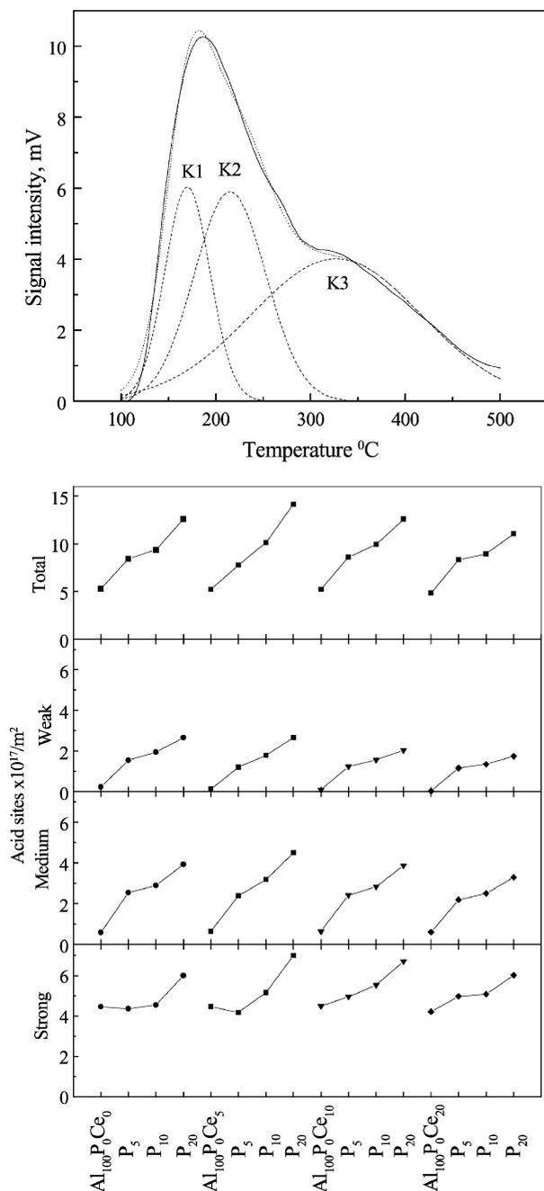
**Fig. 6** Upper part: Deconvolution of a typical NH<sub>3</sub> TPD signal from Fig. 4 (sample Al<sub>100</sub>P<sub>20</sub>Ce<sub>0</sub>). The K<sub>1</sub>, K<sub>2</sub> and K<sub>3</sub> components correspond to weak, medium and strong acid sites respectively. Their development as a function of the composition of the solids is shown in the lower part, which also includes the total number of sites.
