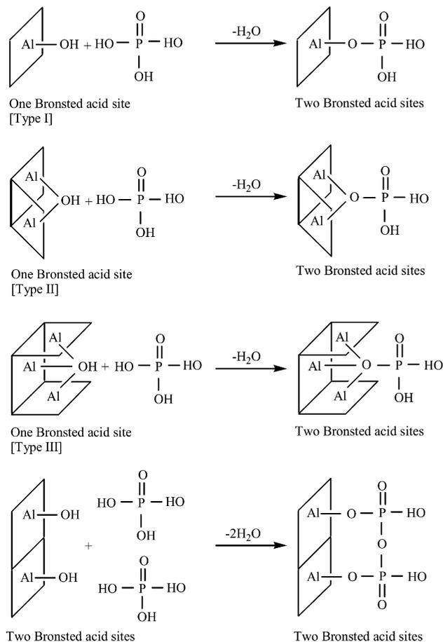
**Fig. 7** Possible schemes for the increase in acid sites in alumina upon addition of phosphate groups.
