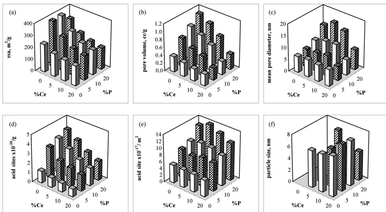
Fig. 3 Variation of the specific surface area (a), the pore volume (b), mean pore diameter (c), the surface acidity of the Al-P-Ce-O solids per g (d) and per m<sup>2</sup> (e) as well as the size of CeO<sub>2</sub> crystallites (f) calculated *via* the Sherrer relationship.
