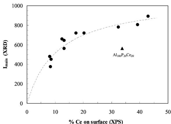
**Fig. 9** Variation of the relative intensity of  $\text{CeO}_2$  main peak ( $I_{\text{main}}$ ) from XRD data (Fig. 1) over the intensity of the main peak for the sample  $\text{Al}_{100}\text{P}_0\text{Ce}_{20}$  ( $I_{\text{main,max}}$ ) with the % surface composition of cerium as found by XPS. The dashed line is described by eqn. (6).
