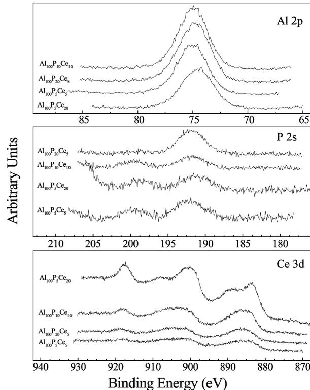
**Fig. 5** Typical XPS spectra for the  $\text{Al}_{2p}$ ,  $\text{P}_{2s}$  and  $\text{Ce}_{3d}$  shells in the  $\text{Al}_{100}\text{P}_x\text{Ce}_y$  solids.
