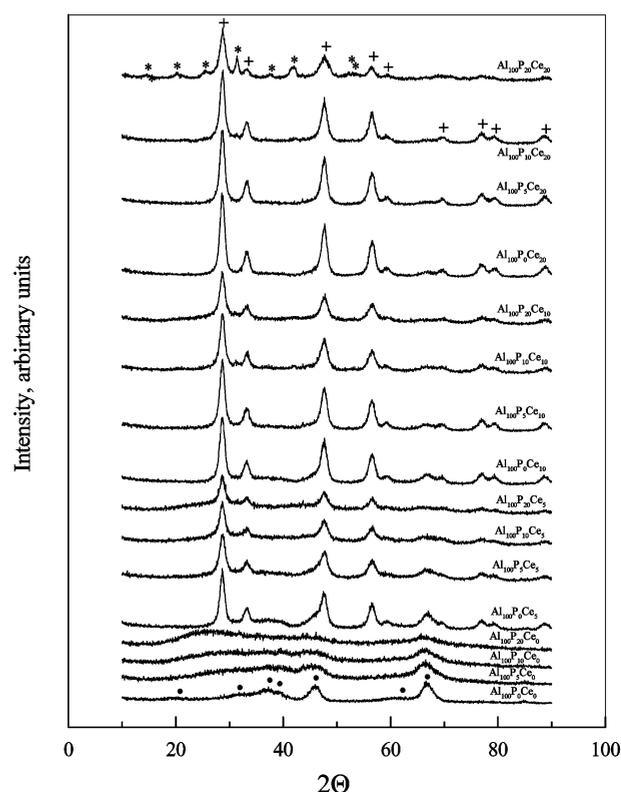
**Fig. 1** XRD patterns of the Al–P–Ce–O mesoporous solids heated at 600 °C. (●)  $\gamma\text{-Al}_2\text{O}_3$ , (+)  $\text{CeO}_2$ , (\*)  $\text{CePO}_4$ .
